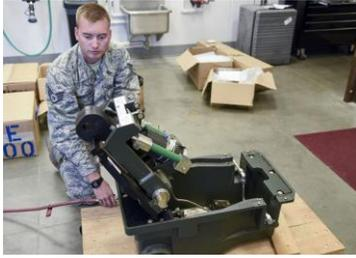
**170909-Z-LQ671-011:** Staff Sgt. Scott Krogstad, 114th Civil Engineer power production specialist, demonstrates the functions of the BAK-14M retractable hook cable support system in the power production shop at Joe Foss Field, Sept. 9, 2017. The support arm and cover assembly of the support box can be raised to a fully open position to give access to the components for servicing. (U.S. Air National Guard photo by Tech. Sgt. Luke Olson)
